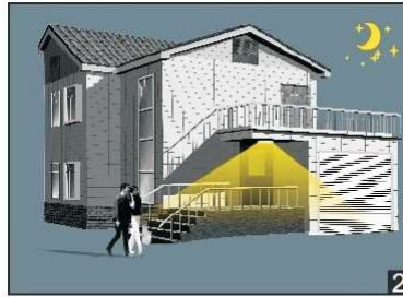
With insufficient daylight, even when motion detected. Light ON.
